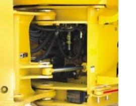
The articulation area opens up, providing easy access to the hydraulics. Centralized lube banks provide better access to all grease zerks to ensure they receive regular service.
