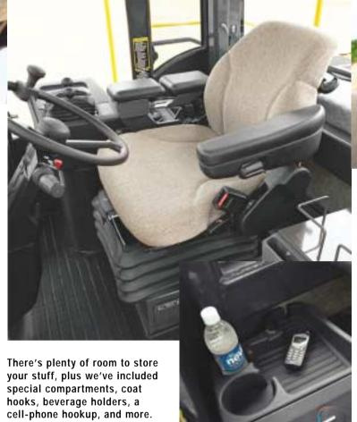
Operators come in all shapes and sizes, which is why the deluxe suspension armchair seat adjusts seven ways, including operator weight, seat cushion angle, backrest angle, and fore and aft.
