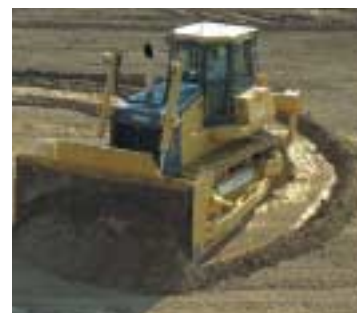
Unlike dozers with differential steering, the highly maneuverable 950C makes tight turns at any travel speed.
