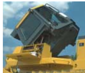
Cab can be tilted in minutes for easier access to the hydrostatic pumps and the engine.
